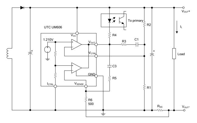
$$V_{OUT} = V_{REF} \times \frac{R1 + R2}{R1} - (I_L \times R_{SS}) \quad (V)$$
