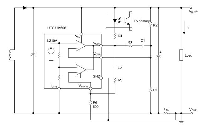
$$V_{OUT} = \left[V_{REF} + \left(I_L \times R_{SS}\right)\right] \times \frac{R1 + R2}{R1} - \left(I_L \times R_{SS}\right) \quad (V)$$
