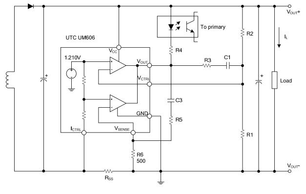
$$V_{OUT} = V_{REF} \times \frac{R1 + R2}{R1}$$
