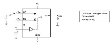
Figure 14. OFF-State Leakage Current (I<sub>NC(OFF)</sub>, I<sub>NO(OFF)</sub>, I<sub>COM(OFF)</sub>, I<sub>NC(PWROFF)</sub>, I<sub>NO(PWROFF)</sub>, I<sub>COM(PWROFF)</sub>)
