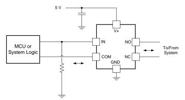
Figure 24. System Schematic for TS5A3160
