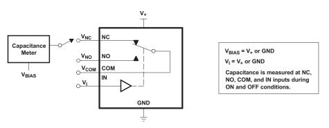
Figure 16. Capacitance (C<sub>I</sub>, C<sub>COM(ON)</sub>, C<sub>NC(OFF)</sub>, C<sub>NO(OFF)</sub>, C<sub>NC(ON)</sub>, C<sub>NO(ON)</sub>)
