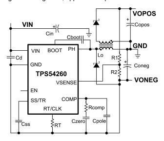
Figure 63. TPS54260 Split-Rail Power Supply based on SLVA369 Application Note
