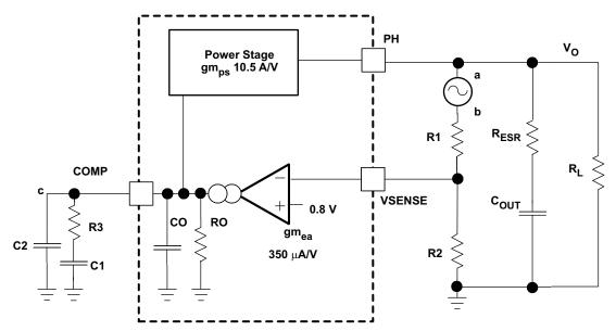
Figure 45. Small Signal Model for Loop Response
