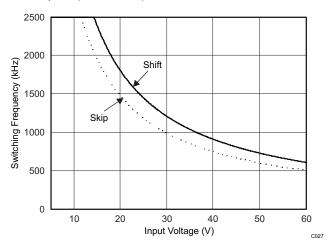
Figure 40. Maximum Switching Frequency vs. Input Voltage
