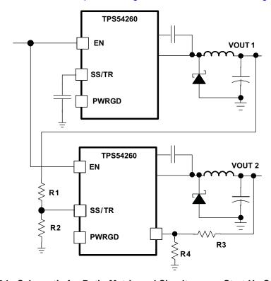
Figure 34. Schematic for Ratio-Metric and Simultaneous Start-Up Sequence
