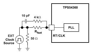
Figure 41. Synchronizing to a System Clock
