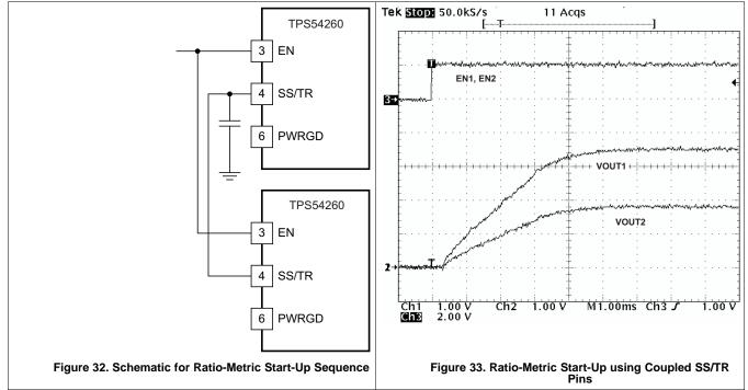
Figure 32 shows a method for ratio-metric start-up sequence by connecting the SS/TR pins together. The regulator outputs will ramp up and reach regulation at the same time. When calculating the slow-start time, the pullup current source must be doubled in Equation 6. Figure 33 shows the results of Figure 32.
