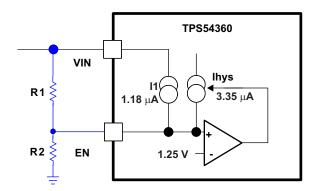
Figure 27. Adjustable Undervoltage Lockout (UVLO)
