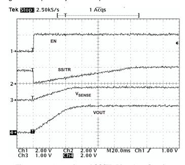
Figure 29. Operation of SS/TR Pin when Starting
