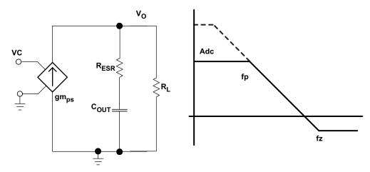
Figure 46. Simple Small Signal Model and Frequency Response for Peak Current Mode Control
