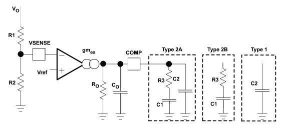
Figure 47. Types of Frequency Compensation
