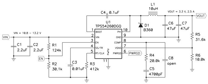
A. The estimated printed circuit board area for the components used in this design is 0.55 inch². This area does not include test points or connectors.
