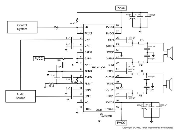
Figure 38. Stereo Class-D Amplifier With BTL Output and Single-Ended Inputs With Power Limiting
