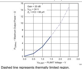
Figure 11. Maximum Output Power vs PLIMIT Voltage (BTL)
