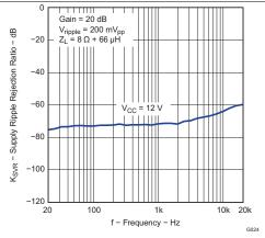
Figure 22. Supply Ripple Rejection Ratio vs Frequency (BTL)
