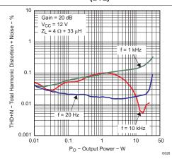
Figure 24. Total Harmonic Distortion + Noise vs Output Power (PBTL)
