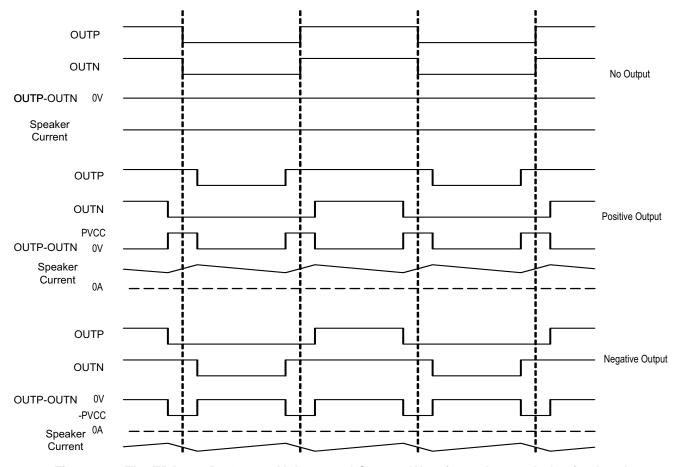
Figure 30. The TPA3113D2 Output Voltage and Current Waveforms Into an Inductive Load
