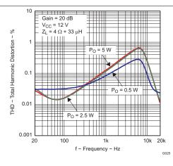
Figure 23. Total Harmonic Distortion vs Frequency (PBTL)
