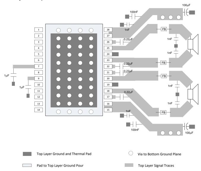
Figure 40. BTL Layout Example
