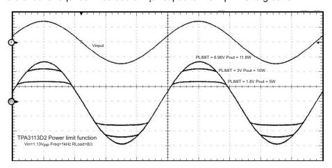
Figure 29. PLIMIT Circuit Operation
