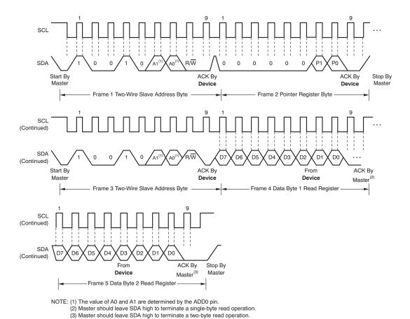
Figure 9. Two-Wire Timing Diagram for Read Word Format
