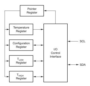
Figure 12. Internal Register Structure
