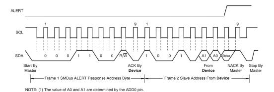
Figure 10. Timing Diagram for SMBus Alert
