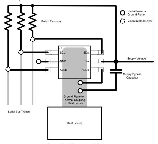
Figure 17. TMP102 Layout Example
