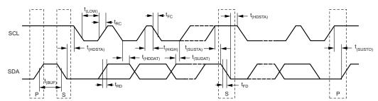
Figure 7. Two-Wire Timing Diagram
