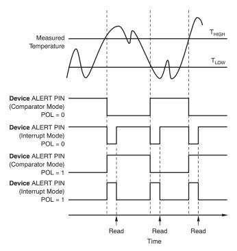
Figure 13. Output Transfer Function Diagrams
