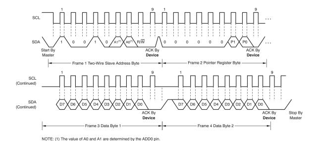
Figure 8. Two-Wire Timing Diagram for Write Word Format
