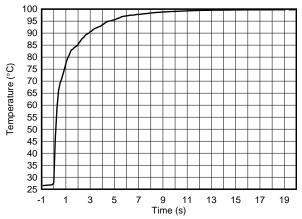
Figure 16. Temperature Step Response
