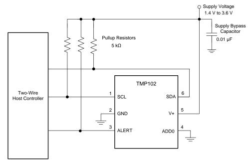
Figure 14. Typical Connections
