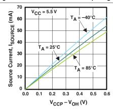
Figure 15. I/O Source Current vs Output High Voltage
