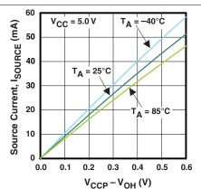
Figure 14. I/O Source Current vs Output High Voltage
