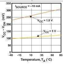
Figure 17. I/O High Voltage vs Temperature
