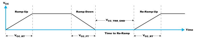
Figure 38.  $V_{CC}$  is Lowered Below 0.2 V or 0 V and Then Ramped up to  $V_{CC}$
