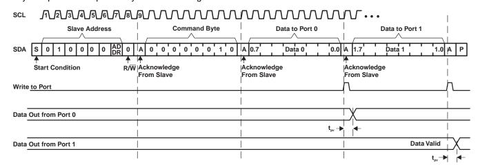
Figure 29. Write to Output Port Register
