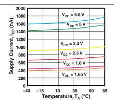
Figure 1. Supply Current vs Temperature
