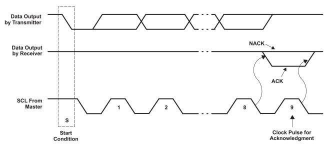
Figure 26. Acknowledgment on the I<sup>2</sup>C Bus
