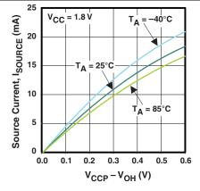
Figure 11. I/O Source Current vs Output High Voltage
