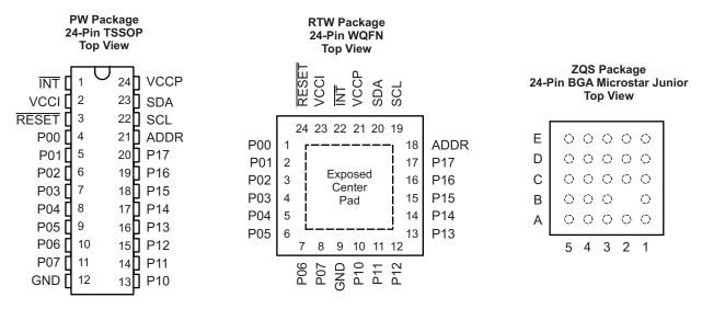
The exposed center pad, if used, must be connected only as a secondary GND or must be left electrically open.
