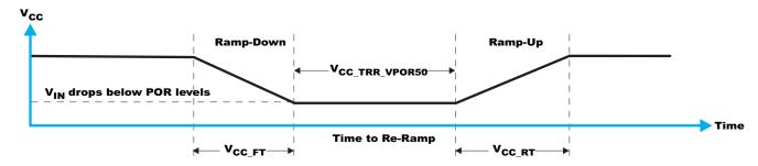
Figure 39. V<sub>CC</sub> is Lowered Below the POR Threshold, Then Ramped Back up to V<sub>CC</sub>
