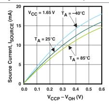
Figure 10. I/O Low Voltage vs Temperature
