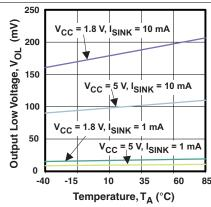
Figure 9. I/O Sink Current vs Output Low Voltage
