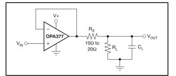
Figure 24. Improving Capacitive Load Drive
