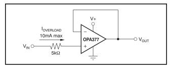
Figure 23. Input Current Protection
