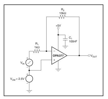
Figure 21. Basic Single-Supply Connection
