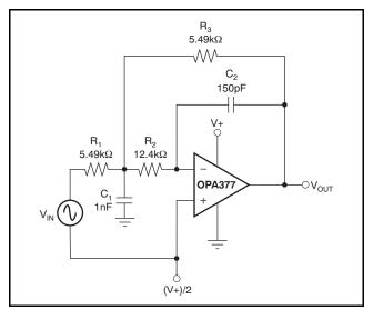
Figure 25. Second-Order Butterworth 50kHz Low-Pass Filter
