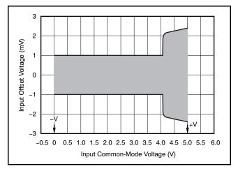
Figure 22. Offset and Common-Mode Voltage
