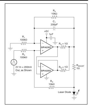
Figure 3. Parallel Operation
