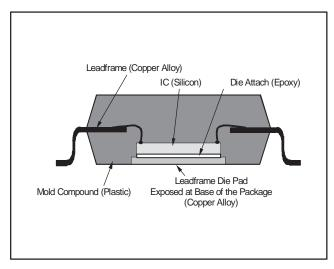
Figure 10. Section View of a PowerPAD Package
