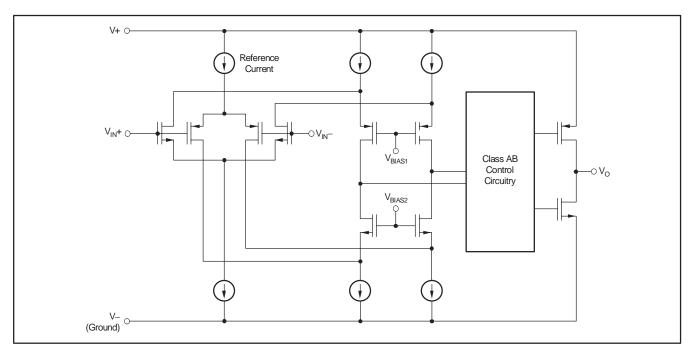
Figure 1. Simplified Schematic
