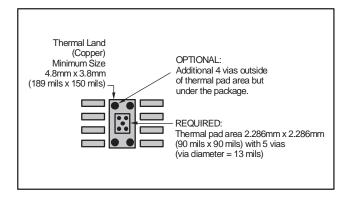
Figure 11. 8-Pin PowerPAD PCB Etch and Via Pattern
