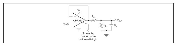
Figure 8. Series Resistor in Unity-Gain Configuration Improves Capacitive Load Drive
