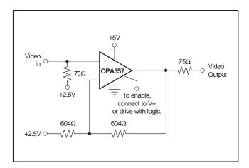
Figure 4. Single-Supply Video Line Driver
