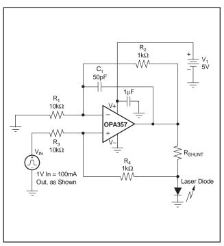
Figure 2. Laser Diode Driver
