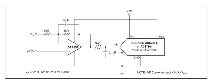
Figure 7. The OPA357 in Inverting Configuration Driving an A/D Converter
