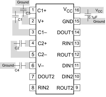
Figure 9. Layout Diagram
