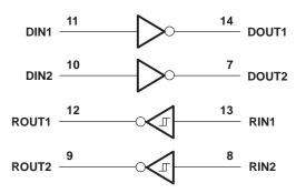
Figure 6. Logic Diagram
