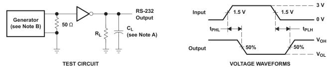
A. C<sub>L</sub> includes probe and jig capacitance
