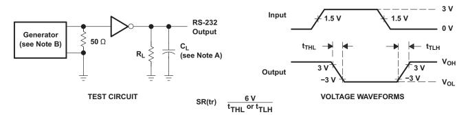
A.  $C_L$  includes probe and jig capacitance
