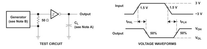
A.  $C_L$  includes probe and jig capacitance
