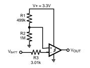
Figure 32. Battery-Sense Application
