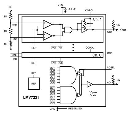
Figure 33. External Resistor Dividers
