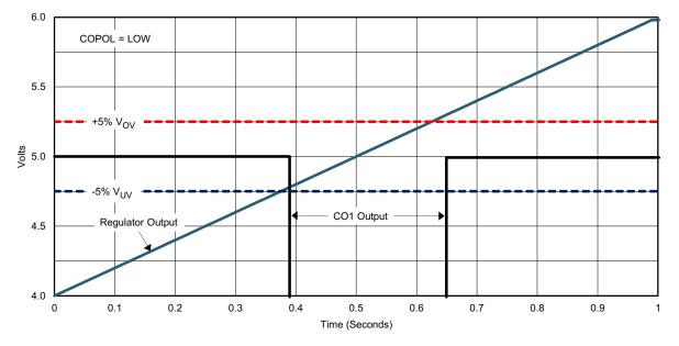
Figure 39. Power Supply Supervisor Thresholds
