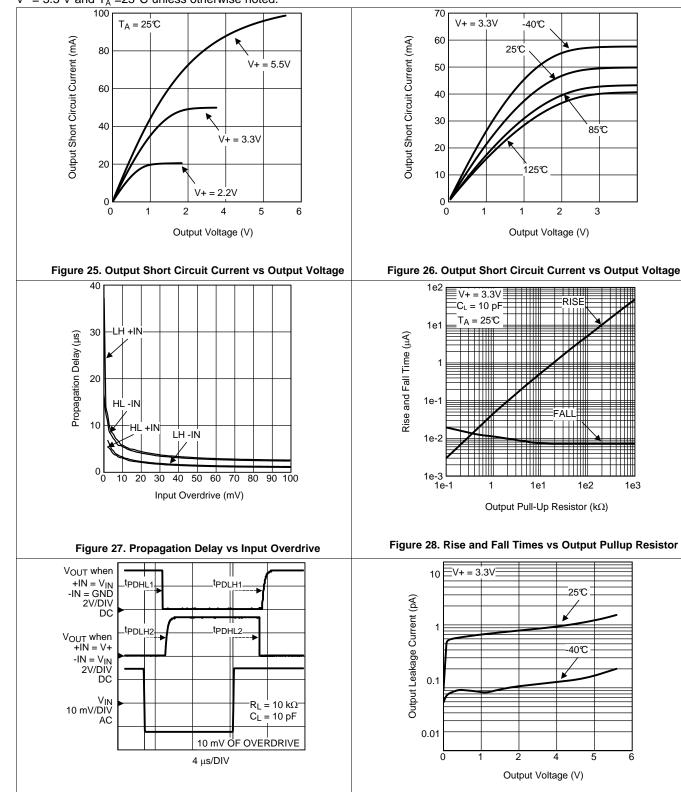
Figure 30. Output Leakage Current vs Output Voltage
