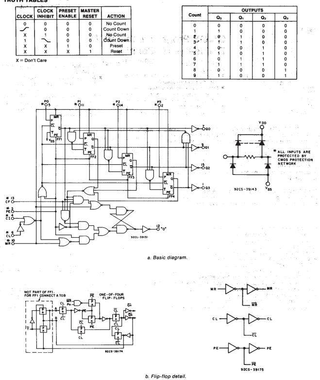
Fig. 1 - Logic diagram for the CD4522B.
