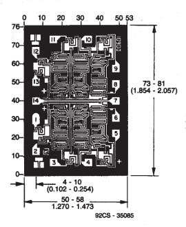
Dimensions in parentheses are in millimeters and are derived from the basic inch dimensions as indicated. Grid graduations are in mils ( $10^{-3}$  inch).
