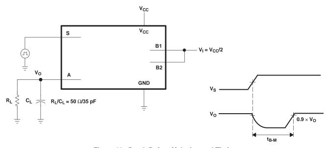
Figure 11. Break-Before-Make Internal Timing
