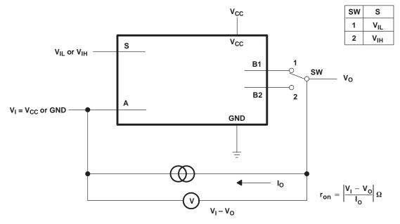
Figure 2. ON-State Resistance Test Circuit
