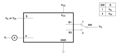
$\begin{array}{l} \text{Condition 1: V}_I = \text{GND, V}_O = \text{V}_{CC} \\ \text{Condition 2: V}_I = \text{V}_{CC}, \text{V}_O = \text{GND} \\ \end{array}$
