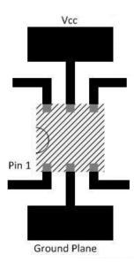
Figure 15. Recommended Layout Example
