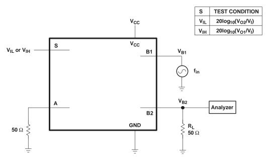
Figure 7. Crosstalk (Between Switches)
