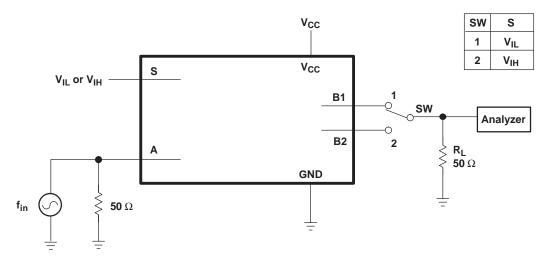
Figure 8. Feedthrough
