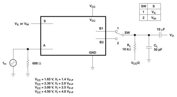
Figure 10. Total Harmonic Distortion
