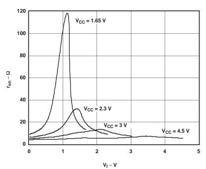
Figure 1. Typical  $R_{on}$  as a Function of Input Voltage (V<sub>I</sub>) for  $V_{I} = 0$  To  $V_{CC}$
