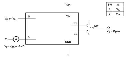
Figure 4. ON-State Switch Leakage-Current Test Circuit
