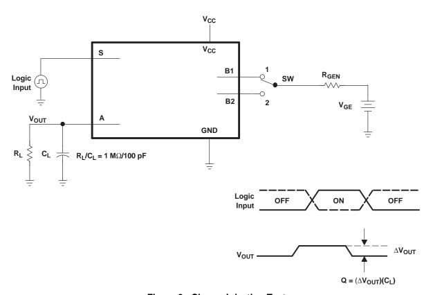
Figure 9. Charge-Injection Test
