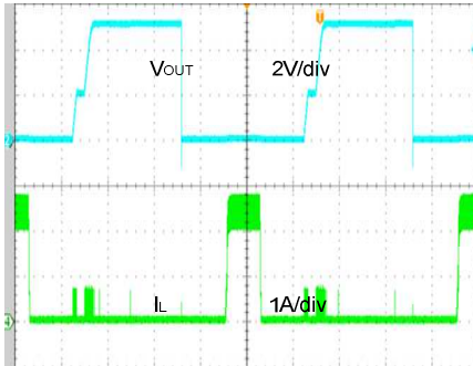
Short Circuit Protection ( V_{IN}=12V , V_{OUT}=5V , 0A to Short)
