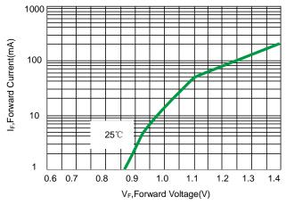
Fig 1. Typical Forward Voltage
