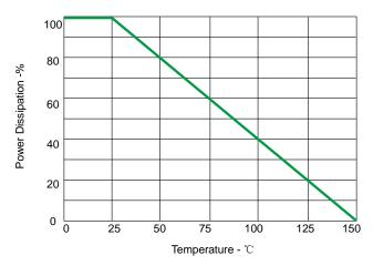
Fig 4.Steady State Power Detating
