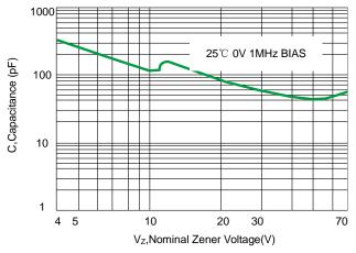
Fig 2. Typical Capacitance
