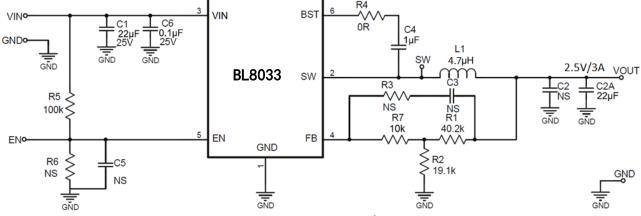
Figure 5. 12V VIN, 2.5V/3A
