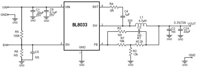
Figure 4. 12V VIN, 3.3V/3A
