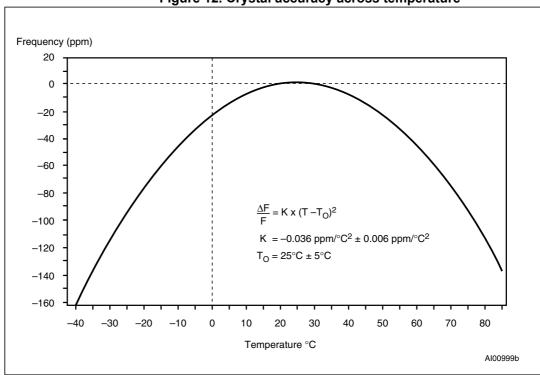
Figure 12. Crystal accuracy across temperature
