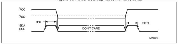
Figure 11. Power down/up mode AC waveforms
