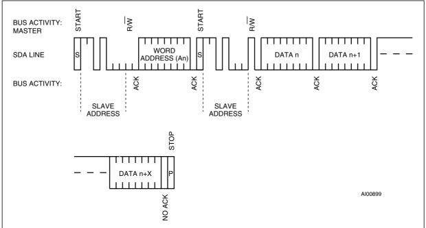
Figure 9. Alternate READ mode sequence
