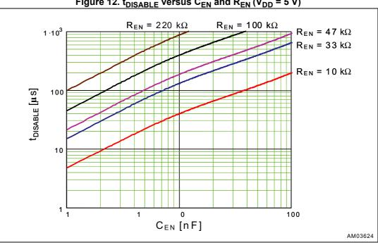
Figure 12.  $t_{DISABLE}$  versus  $C_{EN}$  and  $R_{EN}$  ( $V_{DD}$  = 5 V)
