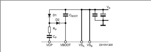
Figure 5. Charge pump circuit
