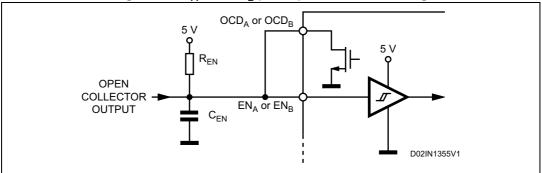
Figure 8.  $\text{EN}_{\text{A}}$  and  $\text{EN}_{\text{B}}$  pins push-pull driving
