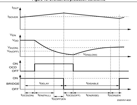
Figure 10. Overcurrent protection waveforms
