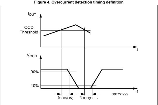
Figure 4. Overcurrent detection timing definition
