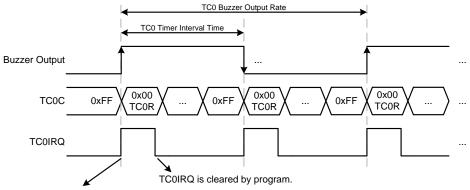
TC0 timer overflows. TC0IRQ set as "1". Reload TC0C from TC0R automatically.
