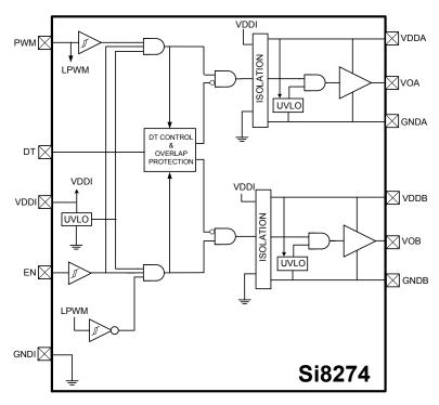
Figure 2.3. Si8274 Block Diagram
