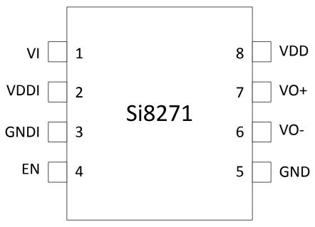
Figure 5.1. Pin Assignments Si8271
