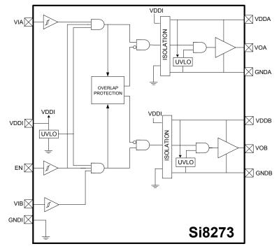
Figure 2.2. Si8273 Block Diagram
