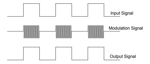
Figure 2.6. Modulation Scheme
