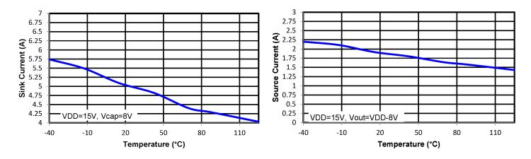
Figure 2.15. Output Sink Current vs. Temperature
