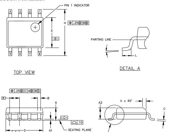
Figure 6.2. 8-Pin Narrow Body SOIC Package
