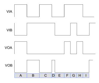
Figure 2.19. Input / Output Waveforms for Si8273 Drivers
