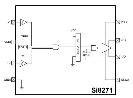
Figure 2.1. Si8271 Block Diagram
