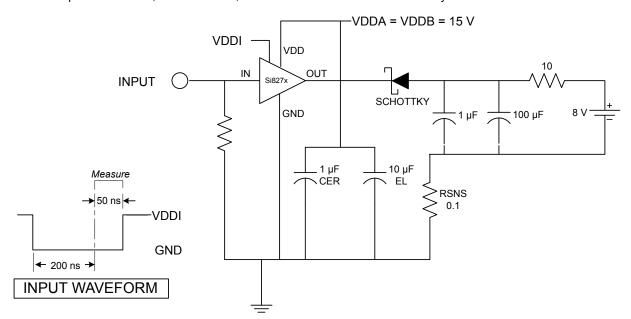
Figure 4.1. IOL Sink Current Test Circuit
