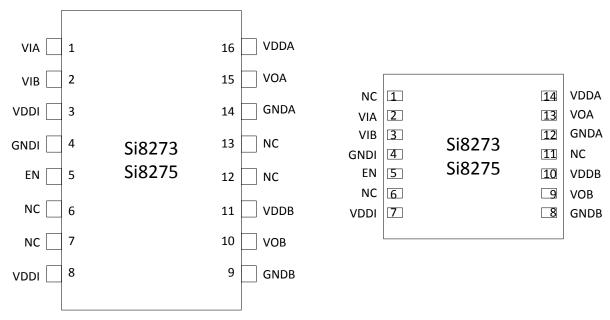
Figure 5.2. Pin Assignments Si8273/5
