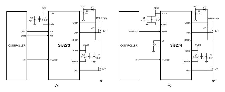
Figure 3.1. Si827x in Half-Bridge Application
