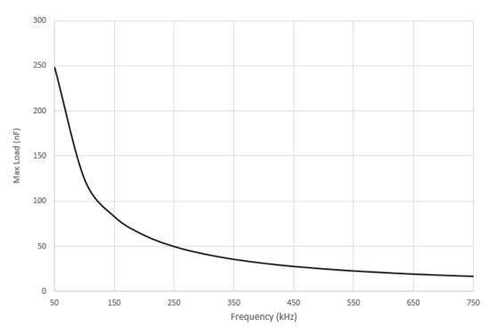
Figure 2.17. Max Load vs. Switching Frequency
