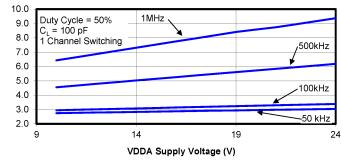
Figure 2.9. Supply Current vs. Supply Voltage
