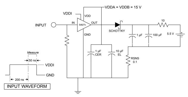
Figure 4.2. IOH Source Current Test Circuit
