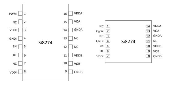
Figure 5.3. Pin Assignments Si8274
