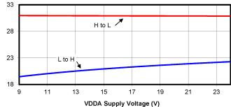
Figure 2.7. Rise/Fall Time vs. Supply Voltage
