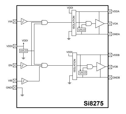
Figure 2.4. Si8275 Block Diagram
