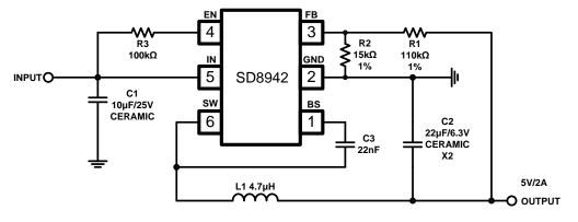
Figure 1. Basic Application Circuit
