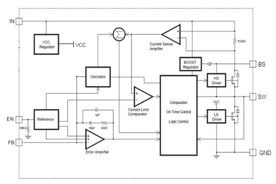
Figure 2. SD8942 Block Diagram
