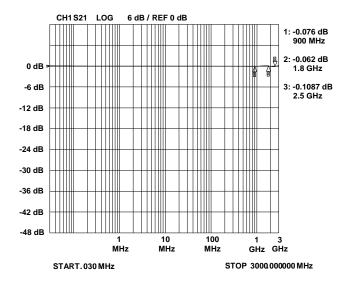
Insertion Loss S21 - I/O to GND
