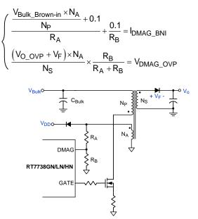
Figure 5. Design DMAG Pin Resistance
