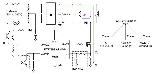
Figure 13. PCB Layout Guide
