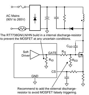
Figure 9. Resistors on Gate Pin
