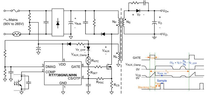
Figure 3. Application Circuit of External Over-Temperature Protection
