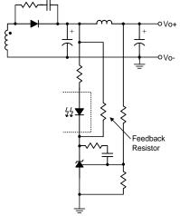
Figure 10. Feedback Resistor
