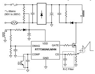
Figure 11. R-C Filter on CS Pin
