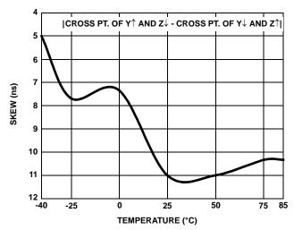
FIGURE 13. DRIVER DIFFERENTIAL SKEW vs TEMPERATURE (ISL3150E, ISL3152E)
