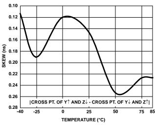
FIGURE 17. DRIVER DIFFERENTIAL SKEW vs TEMPERATURE (ISL3156E, ISL3158E)
