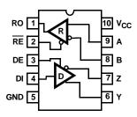
ISL3150E, ISL3153E, ISL3156E (14 LD SOIC) TOP VIEW
