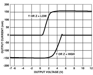
FIGURE 10. DRIVER OUTPUT CURRENT vs SHORT CIRCUIT VOLTAGE
