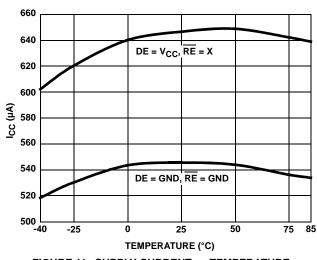
FIGURE 11. SUPPLY CURRENT vs TEMPERATURE
