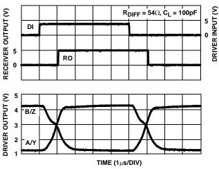
FIGURE 18. DRIVER AND RECEIVER WAVEFORMS, (ISL3150E, ISL3152E)
