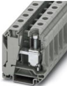
Feed-through modular terminal block, Connection method: Screw connection, Load current : 125 A, Cross section: 10 mm 2 - 35 mm 2 , AWG 8 - 2, Width: 15.1 mm, Color: blue
