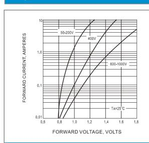
Fig.3 FORWARD CHARACTERISTICS
