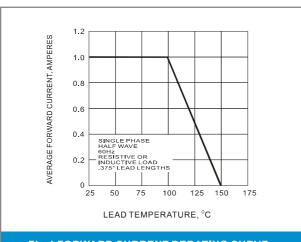
Fig.1 FORWARD CURRENT DERATING CURVE
