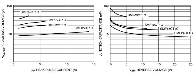
Figure 3. Clamping Voltage vs Peak Pulse Current
