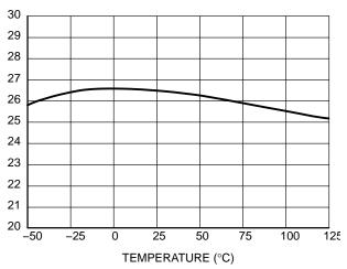
Figure 20. Minimum Switching Frequency fosc(min)
