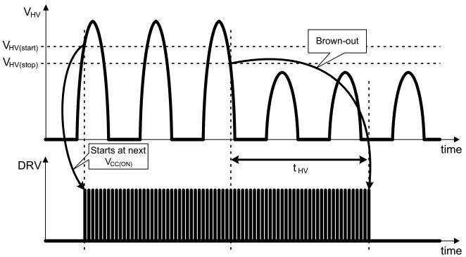
Figure 33. AC Input Brown-out Timing Diagram
