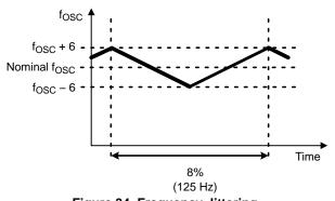
Figure 34. Frequency Jittering
