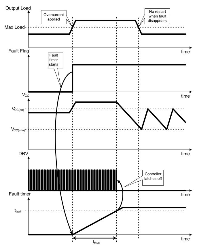
Figure 46. Latched Timer-Based Overcurrent Protection
