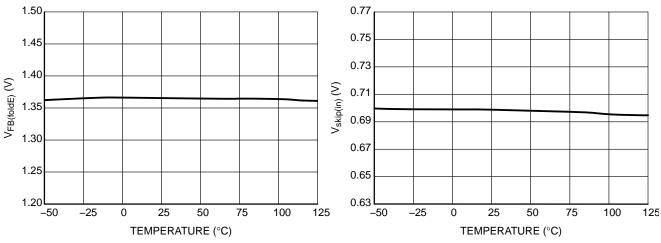
Figure 17. FB Pin Voltage Below Which Frequency Foldback is Complete  $V_{FB(foldE)}$
