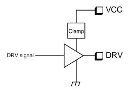
Figure 35. Clamped Driver
