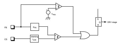
Figure 48. Skip Cycle Schematic
