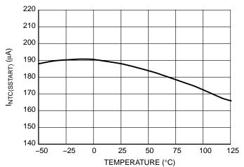
Figure 29. Current I<sub>NTC(SSTART)</sub> Sourced from the Latch Pin, During Soft-Start
