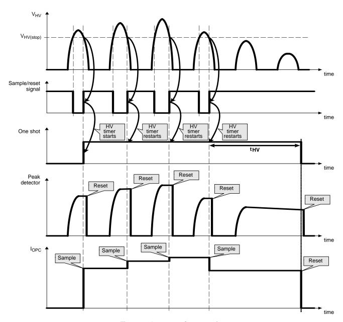
Figure 41. Overpower Compensation
