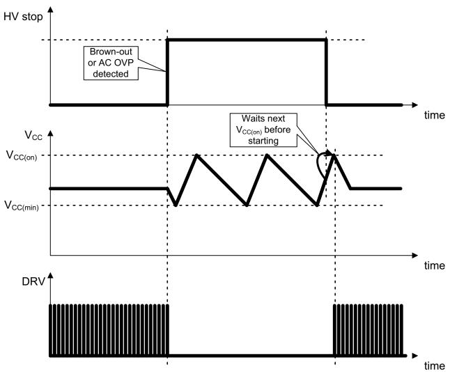
Figure 32. Brown-out Timing Diagram
