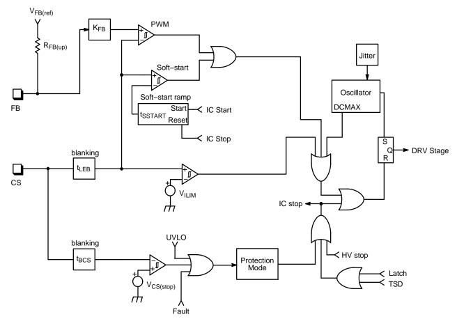
Figure 36. Current Sense Block Schematic
