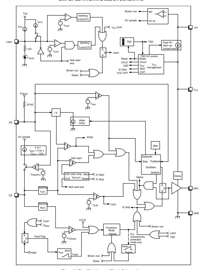
Figure 2. Simplified Internal Block Schematic
