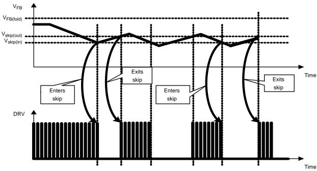
Figure 49. Skip Cycle Timing Diagram
