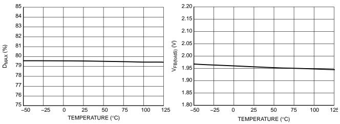
Figure 15. Maximum Duty Cycle  $D_{MAX}$
