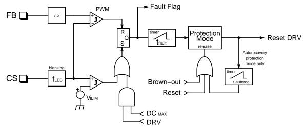
Figure 44. Timer-Based Overcurrent Protection
