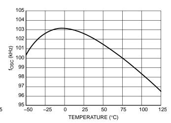
Figure 13. Oscillator Frequency f<sub>OSC</sub> for the 65 kHz version
