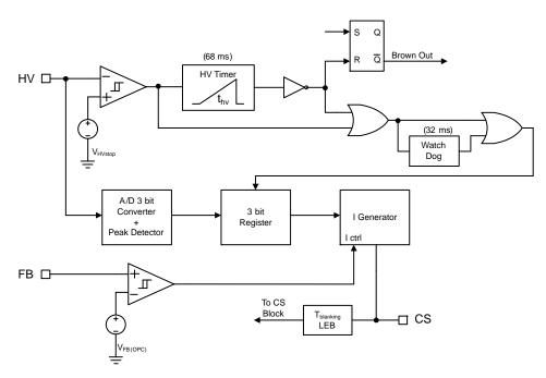
Figure 39. Schematic Overpower Compensation Circuit
