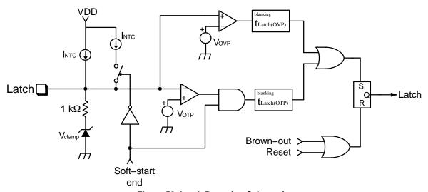
Figure 50. Latch Detection Schematic
