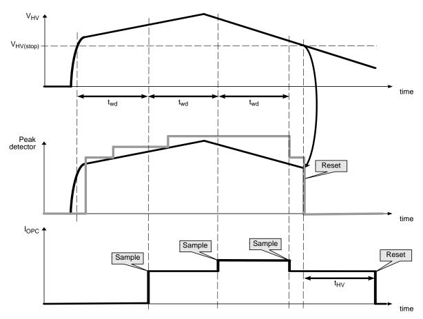
Figure 42. Overpower Compensation
