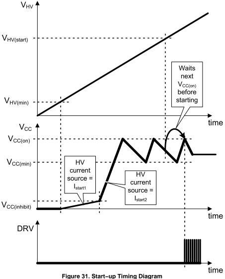
Figure 31. Start-up Timing Diagran
