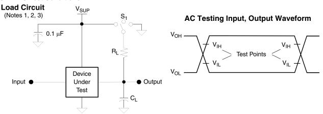
Figure 9. AC Test Conditions,  $T_A = 0^{\circ}C$  to  $70^{\circ}C$ ,  $V_{SUP} = 3.13V - 3.47V$
