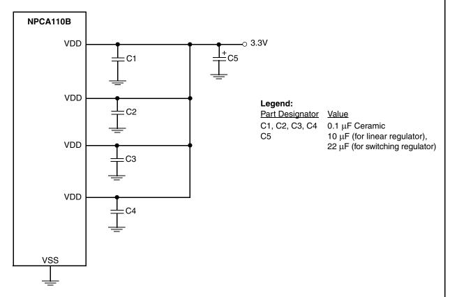
Figure 2. 3.3V Digital Power Connection Diagram
