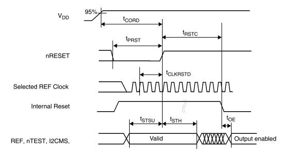
Figure 12. Device Reset
