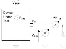
Figure 7. Internal Resistor Test Conditions,  $T_A = 0$ °C to 70°C
