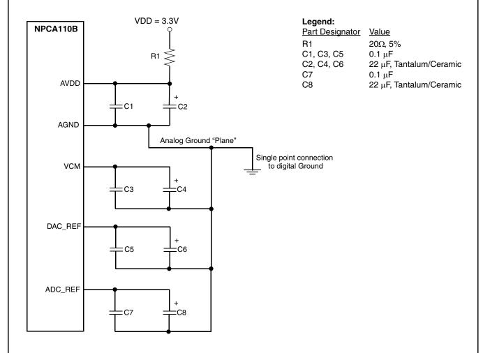
Figure 5. Recommended CODEC Power Connection Diagram
