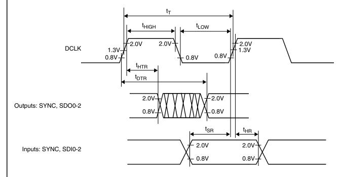
Figure 18. SSI Signal Timing
