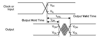
Figure 11. Clock-to-Output and Propagation Delay
