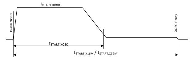
Figure 8 Current drawn at oscillator startup
