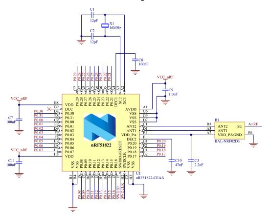
Figure 17 WLCSP with internal LDO regulator
