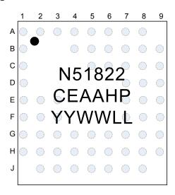
**Figure 3** Ball assignment CEAA packet (top side view)
