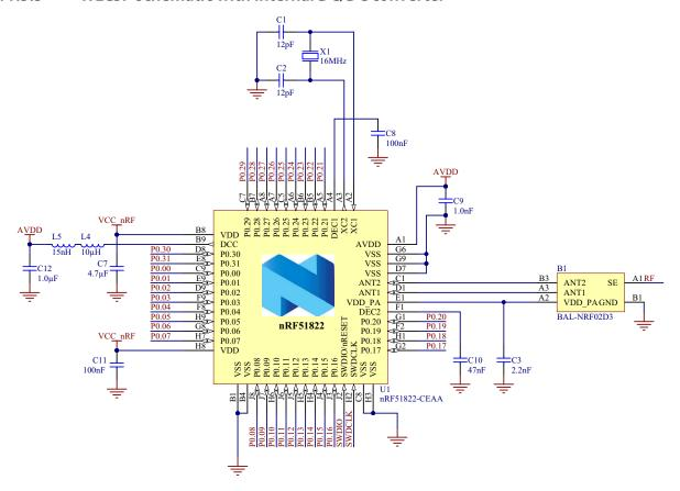
**Figure 19** WLCSP with DC/DC converter
