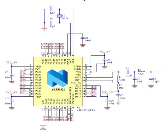
*Figure 15* QFN48 with 1.8 V low voltage mode
