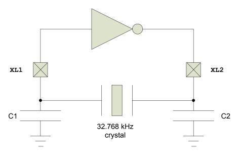
Figure 7 Circuit diagram of the 32.768 kHz crystal oscillator
