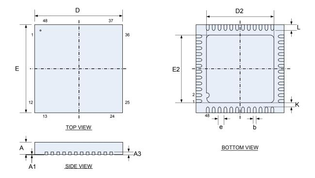
Figure 12 QFN48 6x6 mm package
