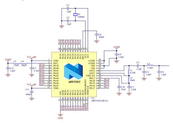
**Figure 16** QFN48 with DC/DC converter
