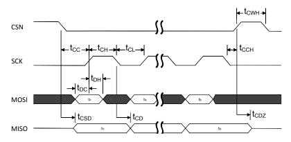
Figure 9 SPIS timing diagram, one byte transmission, SPI Mode 0
