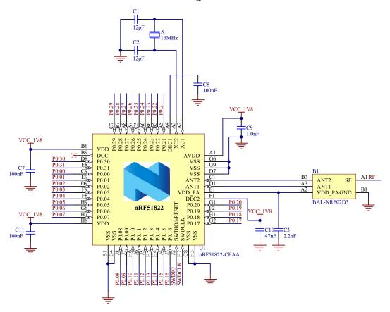
Figure 18 WLCSP with 1.8 V low voltage mode
