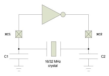
**Figure 6** Circuit diagram of the 16/32 MHz crystal oscillator
