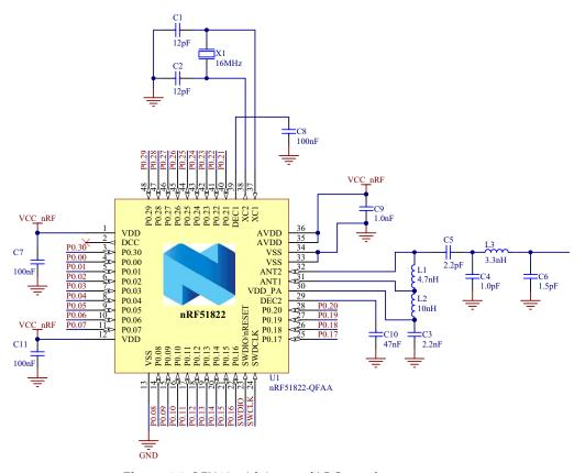
Figure 14 QFN48 with internal LDO regulator
