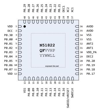
Figure 2 Pin assignment - QFN48 packet
