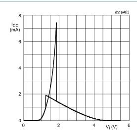
Fig 13. Typical 74AHCT1G14 transfer characteristics;  $V_{CC} = 5.5 \text{ V}$
