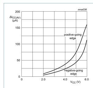
Fig 14. Average additional I<sub>CC</sub> for 74AHC1G14 Schmitt trigger devices; linear change of V<sub>I</sub> between  $0.1V_{CC}$  to  $0.9V_{CC}$
