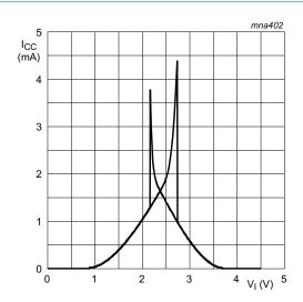
Fig 10. Typical 74AHC1G14 transfer characteristics;  $V_{CC} = 4.5 \text{ V}$
