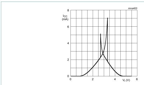
Fig 11. Typical 74AHC1G14 transfer characteristics; V<sub>CC</sub> = 5.5 V
