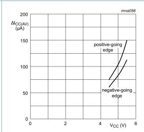
Fig 15. Average additional I<sub>CC</sub> for 74AHCT1G14 Schmitt trigger devices; linear change of VI between  $0.1V_{CC}$  to  $0.9V_{CC}$
