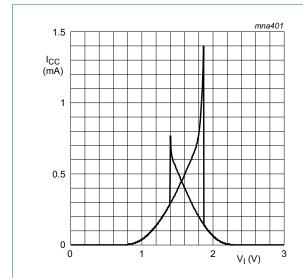
Fig 9. Typical 74AHC1G14 transfer characteristics;  $V_{CC} = 3.0 \text{ V}$
