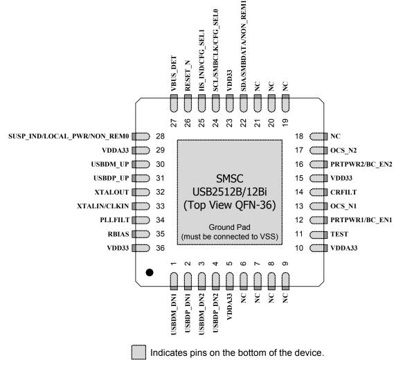
Figure 3.1 2-Port 36-Pin QFN
