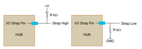
Figure 3.4 Non-Removable Pin Strap Example
