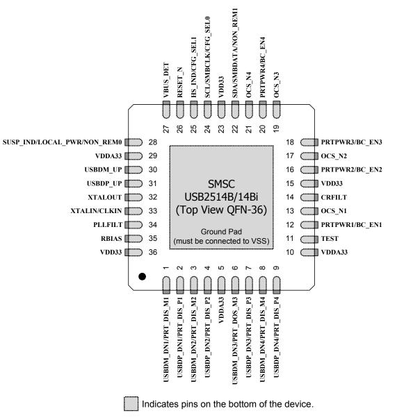
Figure 3.3 4-Port 36-Pin QFN
