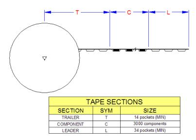
Figure 8.2 36-Pin Package Tape Specifications
