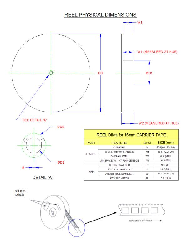
Figure 8.3 36-Pin Package Reel Specifications
