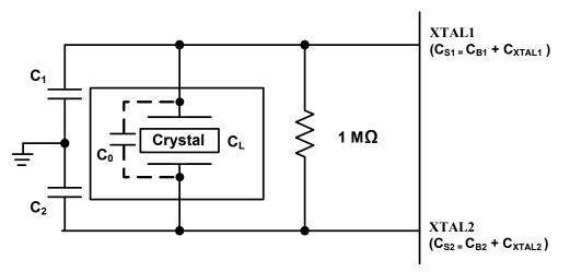
Figure 7.1 Typical Crystal Circuit
