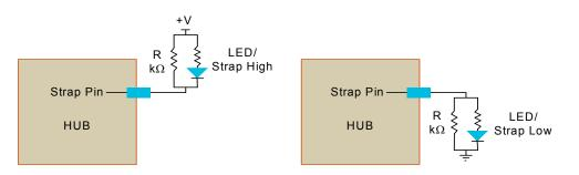
Figure 3.6 LED Pin Strap Example
