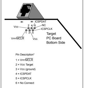
Another connector often found in use with the PICkit<sup>™</sup> programmers is a standard 6-pin header with 0.1 inch spacing. Refer to Figure 28-2.
