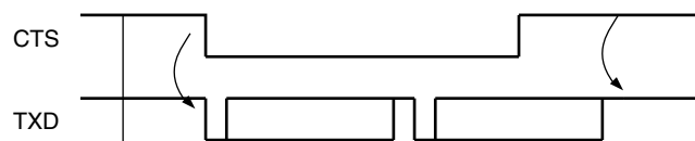
Figure 31-19. Transmitter Behavior when Operating with Hardware Handshaking
