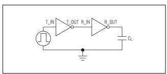
Figure 2. Receiver Test Circuit
