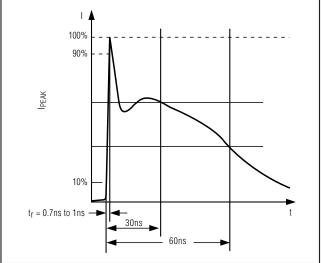
Figure 9b. IEC61000-4-2 ESD Generator Current Waveform
