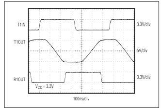
Figure 13. Loopback Test Results at 3Mbps
