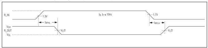
Figure 3. Receiver Propagation Delay
