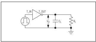
Figure 4. Transmitter Test Circuit
