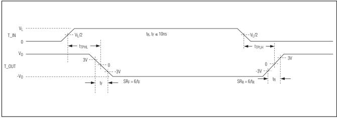
Figure 5. Transmitter Propagation Delay
