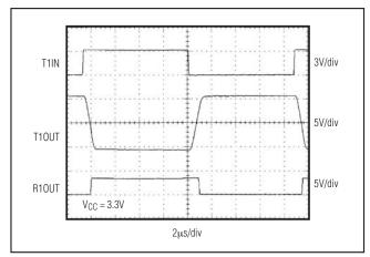
Figure 12. Loopback Test Results at 120kbps
