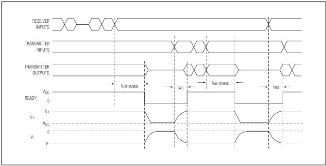
Figure 1. AutoShutdown Plus, and READY Timing Diagram
