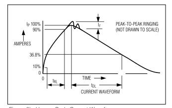
Figure 8b. Human Body Current Waveform
