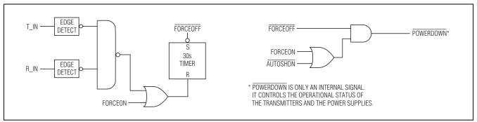
Figure 6. AutoShutdown Plus and Shutdown Logic
