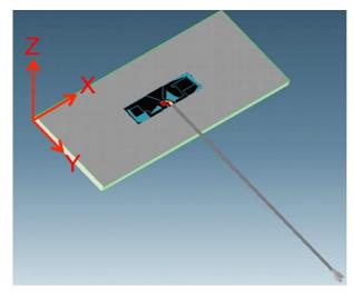
Figure 3a: Antenna on a 1mm-thick PC/ABS material plate
