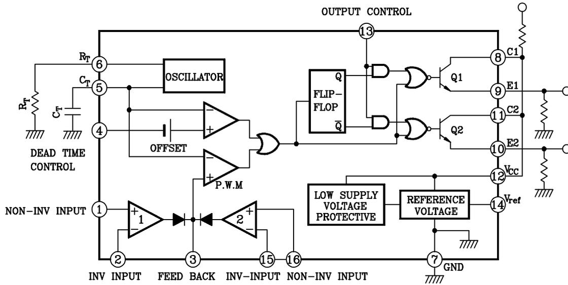
(Note) PIN (13) BECOMES SINGLE MODE AT "L" AND PUSH-PULL MODE AT "H"
