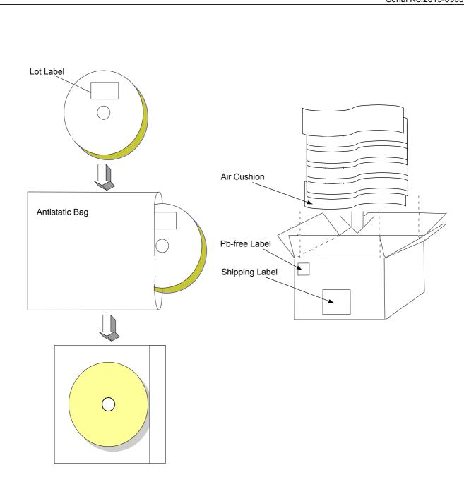
The product is packed up with the method which does not break in the handling by a shipping agent.
