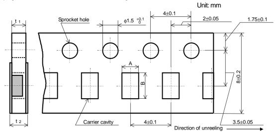
Figure-7 Table-7 Unit: mm Style t<sub>1</sub> t 2 RLC16  $1.9 \pm 0.2$ 1.15±0.15  $0.6 \pm 0.1$ 0.8max. RLC20 1.65±0.15  $2.5 \pm 0.2$  $0.8 \pm 0.1$ 1.0max. RLC32 2.00±0.15  $3.6 \pm 0.2$
