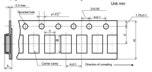
Figure-8 Table-8 Unit: mm Α В W Ε Style t<sub>1</sub> RLC35 3.5±0.05 2.85±0.2  $3.5\pm0.2$ 8±0.3 1.0±0.2 RLC50 3.1±0.2 5.5±0.2 12±0.3 5.5±0.05 1.1±0.15 RLC63  $3.6 \pm 0.2$  $6.9\pm0.2$
