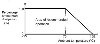
Figure-1 Derating curve
