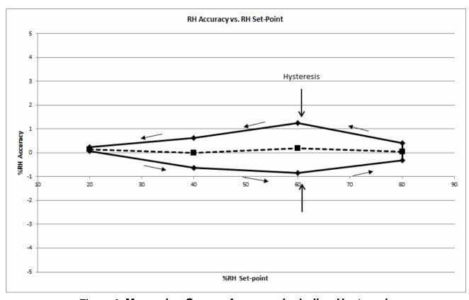
Figure 6. Measuring Sensor Accuracy Including Hysteresis
