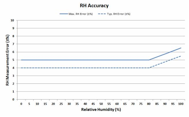
Figure 2. RH Accuracy at 30 °C
