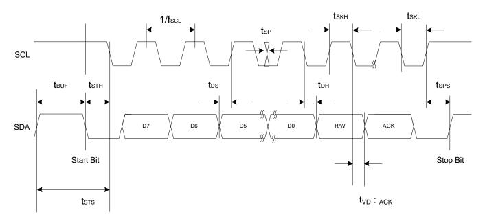
Figure 1. I<sup>2</sup>C Interface Timing Diagram
