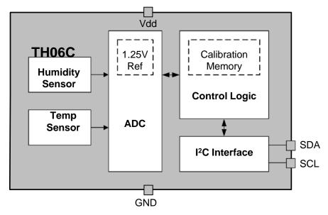
Figure 5. TH06C Block Diagram
