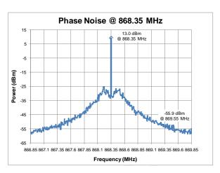
Figure 3. Phase Noise,  $F_{RF}$  = 868.35 MHz,  $P_{OUT}$  = +13 dBm, RBW = 10 kHz, Un-encoded
