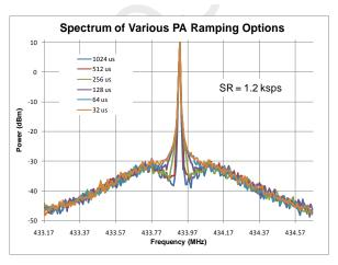
Figure 7. Spectrum of PA Ramping, SR = 1.2 ksps, P<sub>OUT</sub> = +10 dBm
