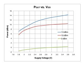
Figure 8. Output Power vs. Supply Voltages,  $F_{RF} = 433.92 \text{ MHz}$
