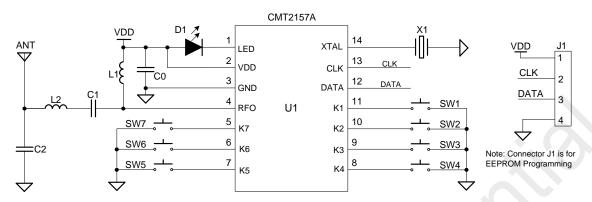
Figure 9. Low-Cost Application Schematic
