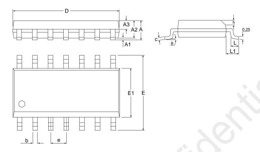
Figure 29. 14-Pin SOP Package
