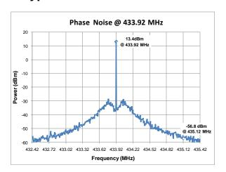
Figure 4. Phase Noise,  $F_{RF}$  = 433.92 MHz,  $P_{OUT}$  = +13 dBm, RBW = 10 kHz, Un-encoded
