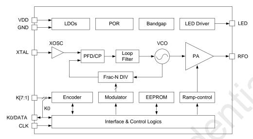
Figure 11. CMT2157A Functional Block Diagram
