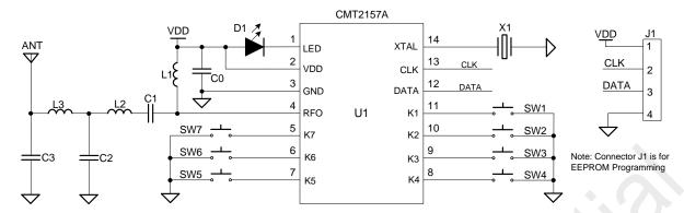
Figure 10. FCC/ETSI Compliant Application Schematic
