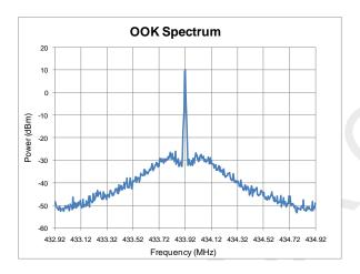
Figure 5. OOK Spectrum,  $P_{OUT} = +10 \text{ dBm}, t_{RAMP} = 32 \text{ us}$
