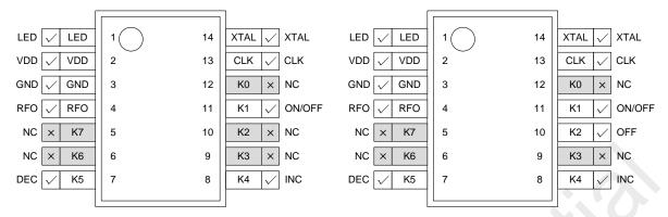
Figure 26. PWM Button Mode with Single (left) and Separated (right) ON/OFF Button(s)
