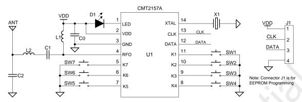
Figure 1. CMT2157A Typical Application Schematic
