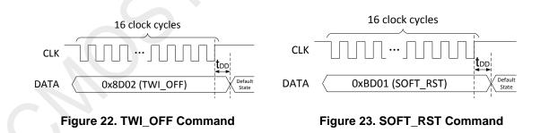
The DATA is generated by the host MCU on the rising edge of CLK, and is sampled by the device on the falling edge. The CLK should be pulled up by the host MCU during the TRANSMISSION shown in Figure 19. The TRANSMISSION process should refer to Figure 16 or Figure 17 for its timing requirement, depending on the "Start By" setting configured on the RFPDK.
