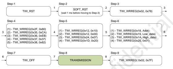
Figure 25. On-line Register Configuration Flow
