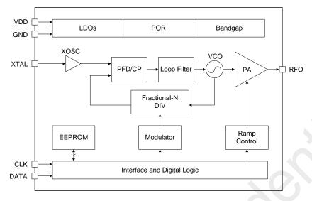
Figure 11. CMT2119A Functional Block Diagram
