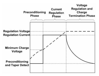
Figure 2: Typical Charge Profile
