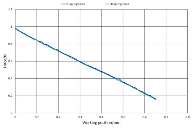
Contact force: 1.0+/-0.3N at working position; Cladding thickness: Au≥0.6um
