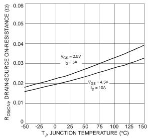
Fig. 6 On-Resistance Variation with Temperature
