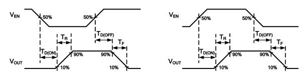
Figure 1. Voltage Waveforms: AP2101 (left), AP2111 (right)
