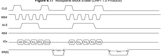
Figure 6.17 Multiplane Block Erase (ONFI 1.0 Protocol)
