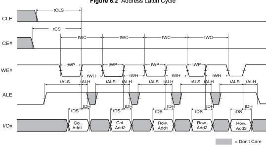
Figure 6.2 Address Latch Cycle
