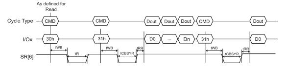
As defined Α for Read CMD CMD ADDR ADDR ADDR ADDR ADDR Dout Dout Cycle Type CMD Dout Page N I/Ox ≺ 30h R1 R2 31h D0 00h C1 Dn tRR tWB tWB tR SR[6] tCBSYR ADDR ADDR ADDR ADDR CMD ADDR Dout Cycle Type Page R 31h D0 I/Ox tRR tWB SR[6] tCBSYR
