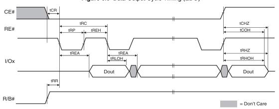
Figure 6.5 Data Output Cycle Timing (EDO)
