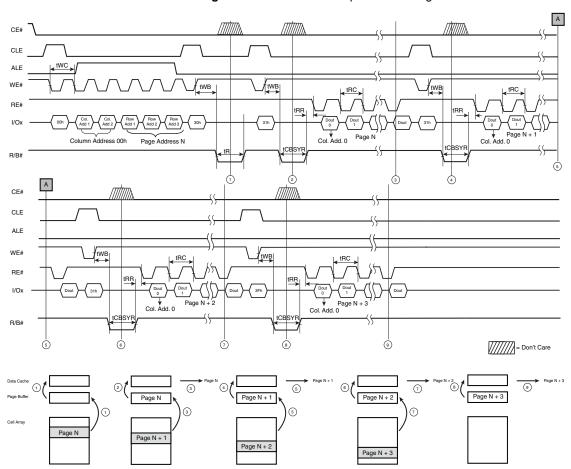
Figure 6.25 Read Cache Operation Timing
