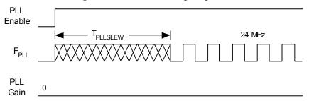
Figure 13. PLL Lock for Low Gain Setting Timing Diagram
