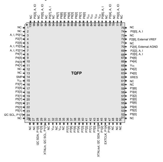
Figure 7. CY8C29866 100-Pin PSoC Device
