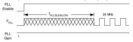
Figure 14. External Crystal Oscillator Startup Timing Diagram
