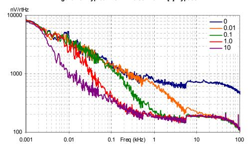
Figure 16. Typical AGND Noise with P2[4] Bypass
