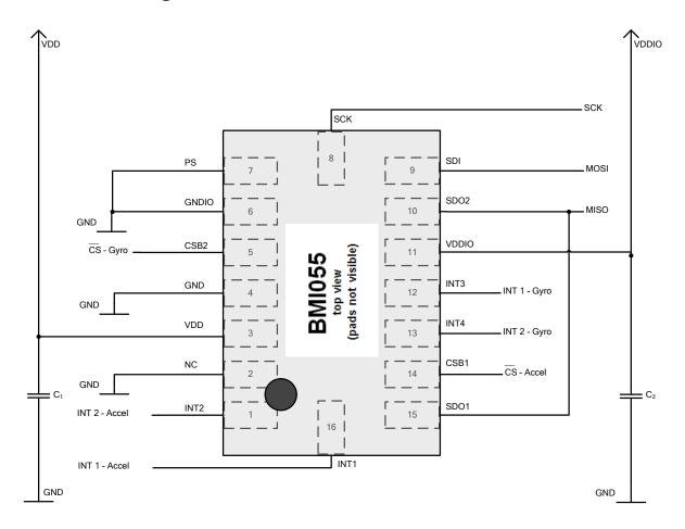
Figure 31: 4-wire SPI connection
