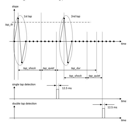
Figure 8: Timing of tap detection
