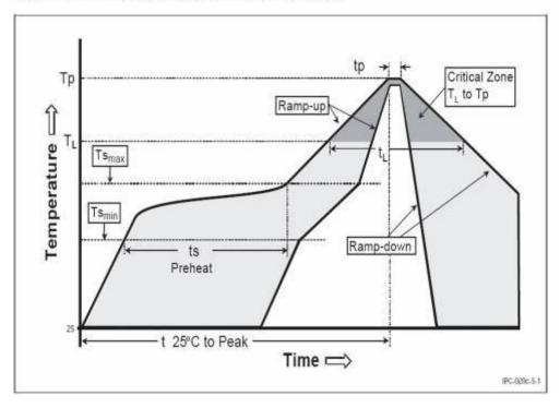
Figure 37: Soldering profile
