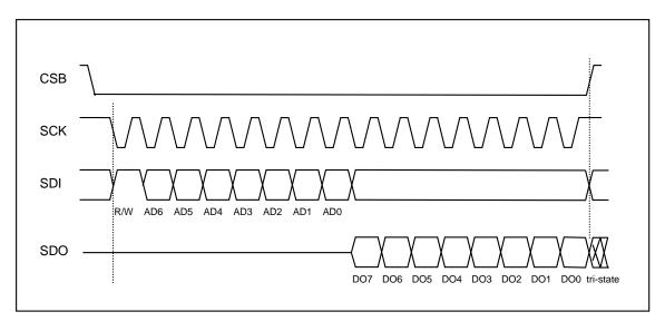
Figure 22: 4-wire basic SPI read sequence (mode '11')
