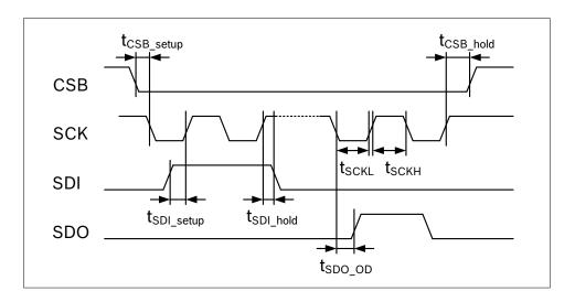
Figure 20: SPI timing diagram
