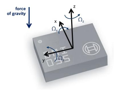
Figure 35: Orientation of sensing axis
