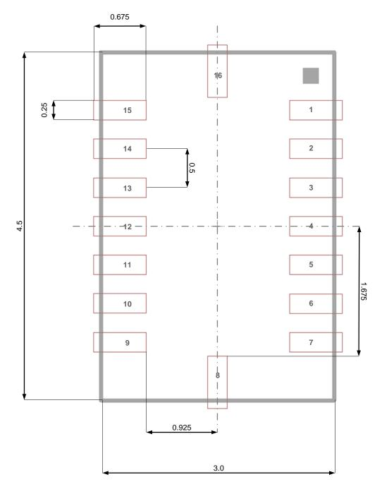
Figure 36: Landing patterns, dimensions are in mm
