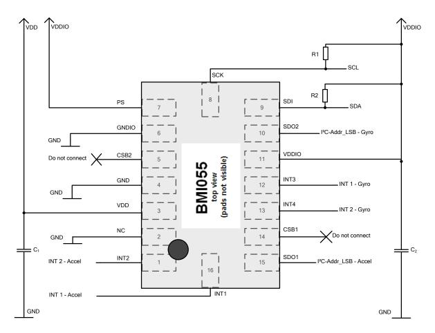
Figure 33: I<sup>2</sup>C connection
