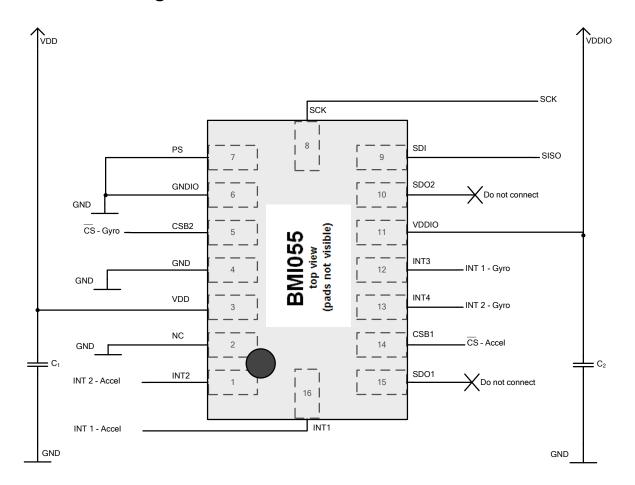
Figure 32: 3-wire SPI connection
