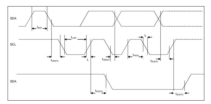
Figure 25: I2C timing diagram
