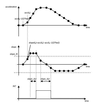
Figure 7: Principle of any-motion detection
