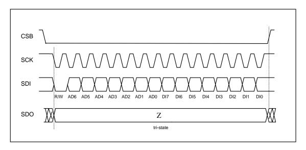
Figure 21: 4-wire basic SPI write sequence (mode '11')
