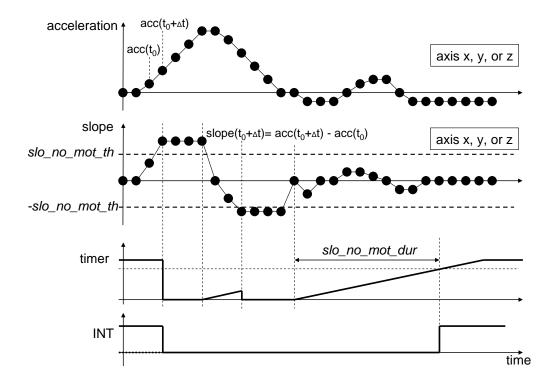
Figure 11: Timing of no-motion interrupt
