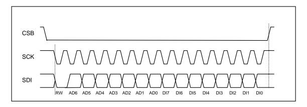
Figure 24: 3-wire basic SPI read or write sequence (mode '11')
