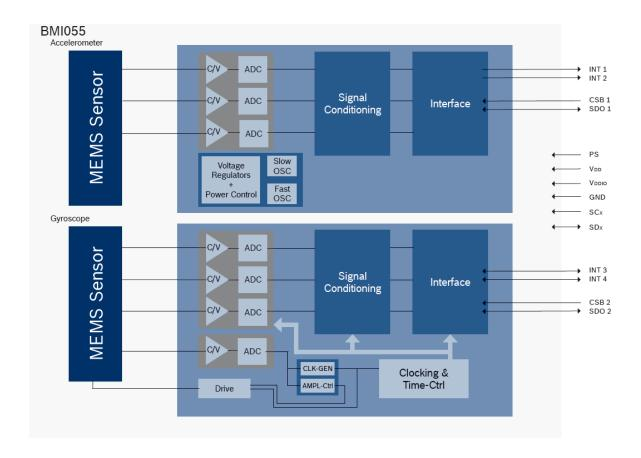
Figure 1: Block diagram of the BMI055
