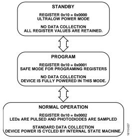
Figure 15. State Machine Operation Flowchart
