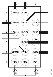
Figure 22. ADPD1080 Connection and PCB Layout Diagram (Top View)
