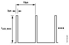
Figure 24. Typical LED Pulse Burst Sequence Configuration
