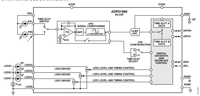
Figure 1. Block Diagram for the ADPD1080
