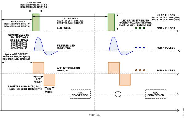
Figure 18. AFE Operation Diagram
