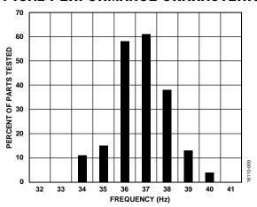
Figure 5. 32 kHz Clock Frequency Distribution (Default Settings, Before User Calibration: Register 0x4B = 0x2612)
