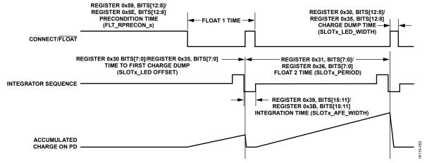
Figure 36. Example of Float Ambient Mode Timing
