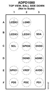
Figure 4. Pin Configuration
