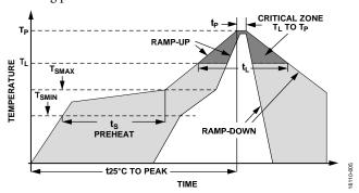
Figure 3. Recommended Soldering Profile
