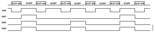
Figure 27. Optional Timing Signals Available on GPIOx—Register 0x0B, Bits[12:8] or Bits[4:0] = 0x02, 0x0C, 0x0D, and 0x0E
