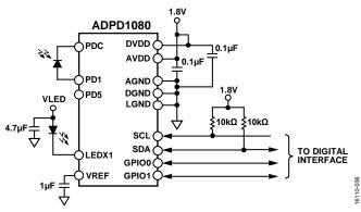
Figure 21. Typical Wrist-Based HRM Measurement
