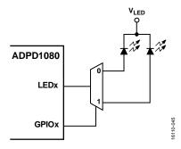
Figure 28. Example Using the f<sub>s</sub>/2 Timing Signal
