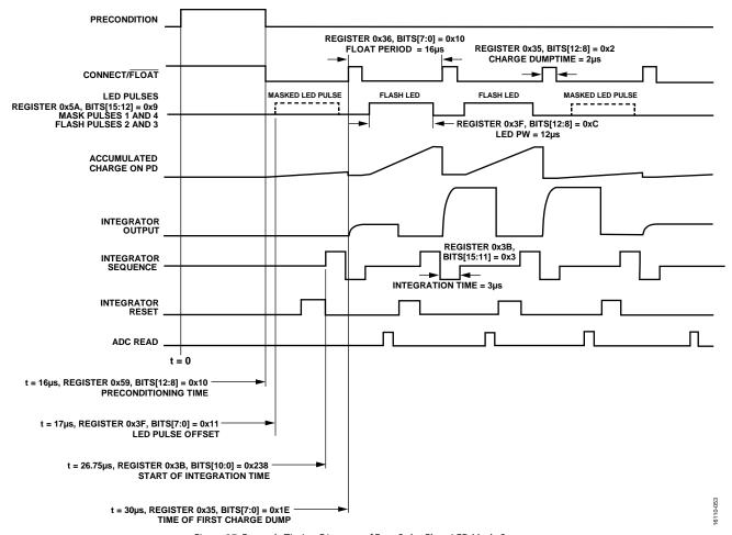
Figure 37. Example Timing Diagram of Four Pulse Float LED Mode Sequence
