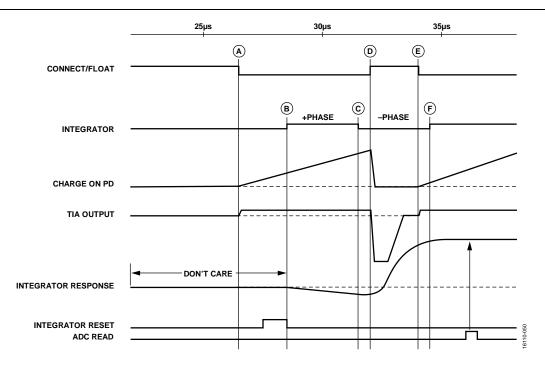
Figure 34. Float Mode Measurement Cycle Timing Diagram
