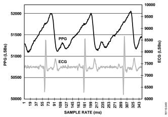
Figure 32. Plot of Synchronized ECG and PPG Waveforms
